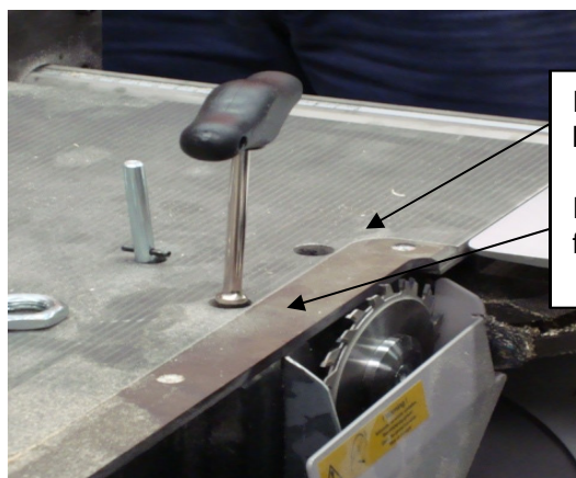
To adjust scribe blade position
